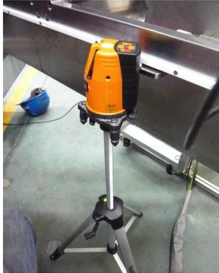
Fig 2: Laser Leveller
