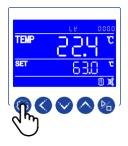
• Press the SETTING key once entering the required code for the parameter level you want to change.
