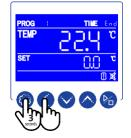
• Press the SETTING and SHIFT keys for 3 seconds to enter the controller's internal parameter settings. The Time area will change and first digit will blink.
