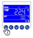
• Press the SETTING key 2 times to set parameter Cy and return to the multi-step program standard state.
