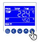
• Press the RUN key for 2 seconds to start the program. STEP area, RUN, HEAT, and run time will illuminate.
