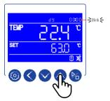
• Press the INCREASE key to enter the first time value. Press the SHIFT key to move to the second time digit. Digit will blink. Press the INCREASE key to enter the second time value.
