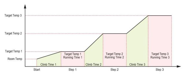
Target temp: The temperature you want it to run as planned (Input/set temperature).
