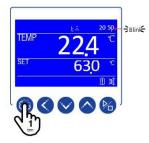
• The tM parameter will appear. Press the SETTING key 1 time to scroll through parameters until the parameter Po appears.
