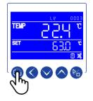
• Press the SETTING key to enter the Level 2 controller parameters.
