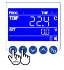
• Press the SETTING and SHIFT keys for 3 seconds to enter the controller's internal parameter settings. Time area will change and first digit will blink.
